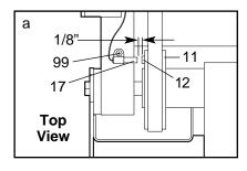
Screw (99) and move the Reed Switch slightly. Retighten the Screw. Re-attach the hood and run the treadmill for a few minutes to check for a correct speed reading.
